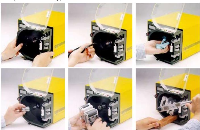
To remove the track, remove any tubing from the pumphead. Loosen the rotor securing bolt and give the rotor/bolt a sharp tap to free the collet. Release the collet, and withdraw the rotor from the shaft. Loosen the two track securing screws and pull the track clear. Use this method of removal and fitting in case cleaning is required.
