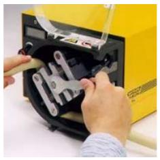
Fit the other end of the tube into the top adjustable clamp, ensuring that the tube is not slack in the pumphead since this can reduce tube life. Clamp the tube very firmly by turning the upper serrated adjustment wheel. Remove the spanner and close the guard.
