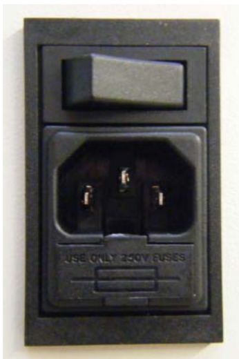
Main switch and fuse holder in the backside
