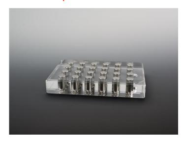
Ideal for DNA purification using standard 2,0 ml deep well plates with round bottom.
